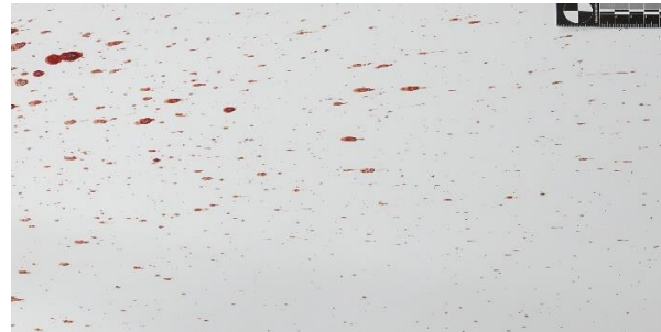
Figure 8, A pattern created by a mechanism (rubber hammer) that struck a bloody ice hockey puck. Different directions of the blood drops with different sizes can be recognised. Energy direction is from left to right.
