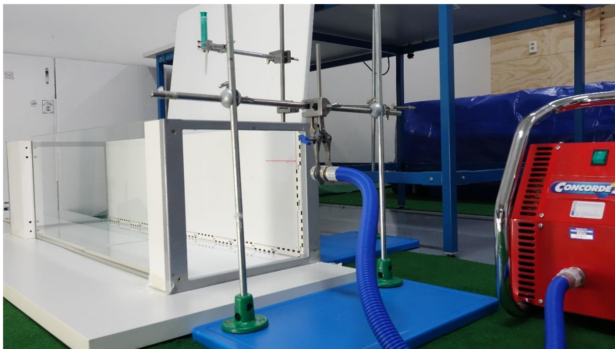
Figure 4, Setup for Blood droplet experiment. On the right is the compressor placed in to a stand with a fixed mechanism. The wind is blown into the wind tunnel of different distances to imitate the correct wind force. Blood drops are release from the pipette, which will follow a trajectory in the wind tunnel. The wind tunnel has a maximum distance of 180 centimetres with a vertical rigging behind it where blood drops can be collected on a white background. The needle can be replaced by three other pieces that vary in volume.
